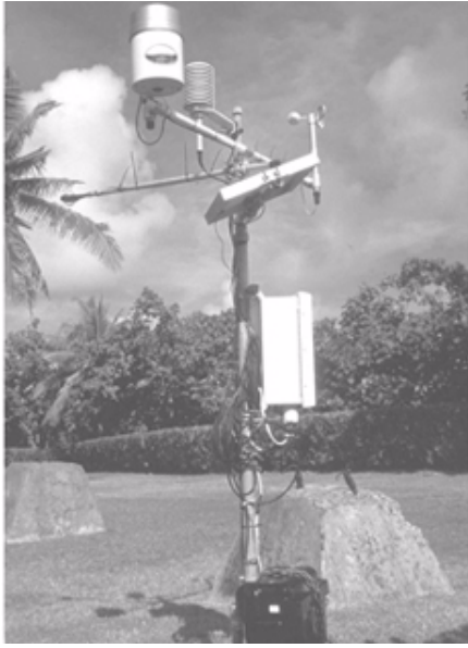
Figure 2. Evapotranspiration station at the SMO Observatory on Tutuila, American Samoa.
