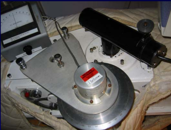
Mercury Lamp in place
