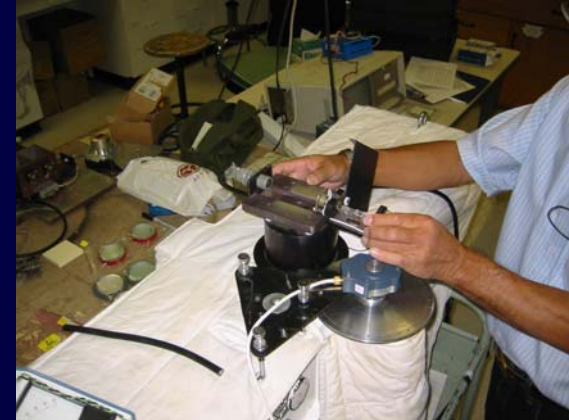
Slide into lamp holder touching only the lamp base
