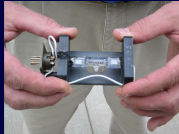
Always hold the lamp from the base
