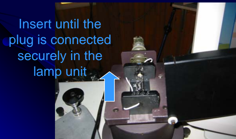
The lamp holder needs to be in place over the GQP before sliding the lamp in
